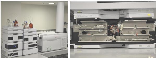
**LC:** Agilent 1200 series comprising of two degassers, two binary pumps, an auto sampler and a column compartment containing a 10-port 2-position valve (a minimum of 8 ports are required)
