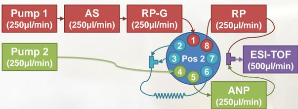
Molecules are eluted off the columns by sequential gradients from each pump, before equilibrated for the next run.
