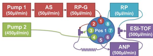
**Resolving steps:** the valve is switched to allow solvent from Pump 1 to flow through the RP-G then the RP analytical column, whilst solvent from Pump 2 flows onto the ANP. Eluant from both columns is mixed before directed to the MS.
